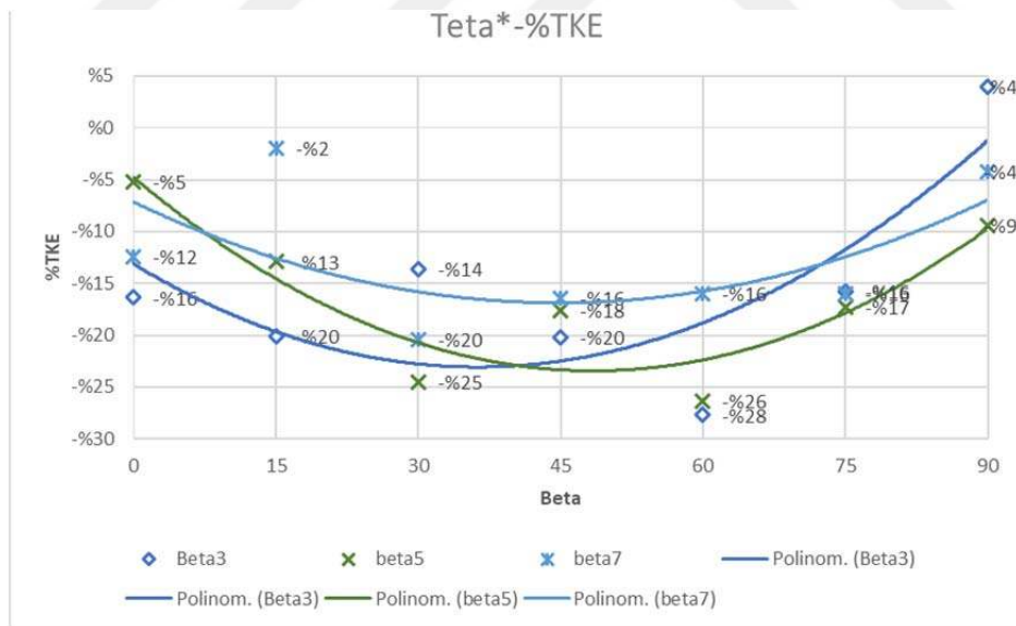
Figure 4.61. TKE variation due to different rotation angle values of 0,15,30,45,60,75 and 90 degrees for porosity values ( \beta ) of 0.3, 0.5, 0.7. Splitter plate ( ls^* ) is 1. Gap between splitter plate midpoint and cylinder ( lg^{**} ) is 1.5.
