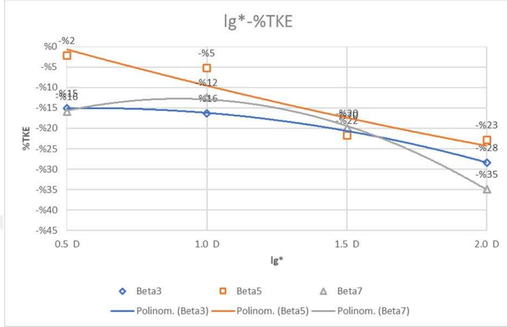
Figure 4.20. TKE var. due to different gaps between the cylinder and leading edge of splitter plate ( lg^* ) for porosity \beta=0.30, 0.50, 0.70 . Splitter plate length ( ls^* ) is 1.
