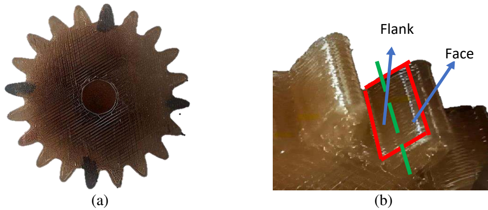
Figure 5.10 (a) Ultem 1010 spur gear, (b) face and flank on the tooth surface
