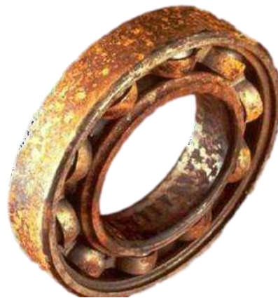
Figure 4.13 Bearing surface damaged by corrosive wear (Aleksandar Vencl et al., n.d.)
