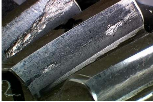
Figure 4.12 Macro pitting failure on gear tooth (Sun et al., 2017)
