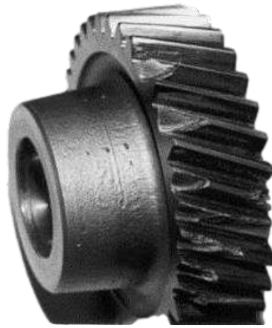
Figure 4.11 Appearance in general of the damaged helical gear (Asi, 2006)
