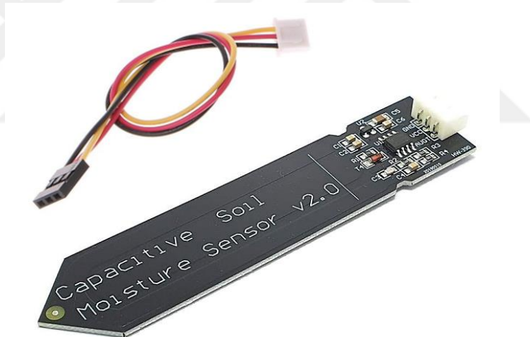
Figure 3.2. Capacitive Soil Moisture v2.0 [42]
