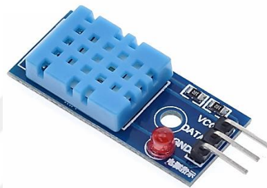
Figure 3.4. Air Temperature and Humidity Sensor (DHT11) [45]
