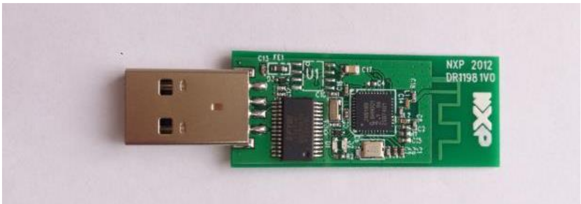
Figure 2.16. Receiver device (NXP JN5169)
