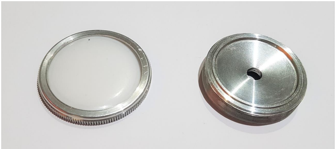
Figure 2.12. Diaphragm and chest piece of the electronic stethoscope
