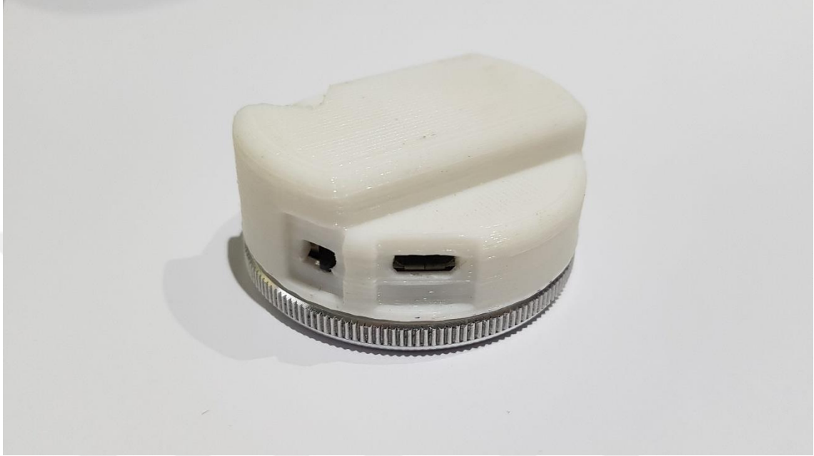
Figure 2.11. IoT-driven electronic stethoscope
