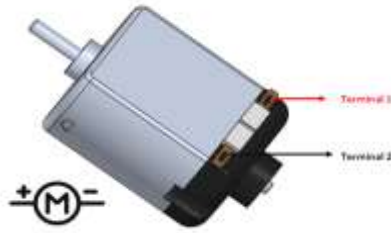
Figure 3.6: Toy DC Motor Wiring.
