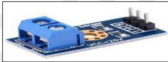
Figure 3.7: DC Voltage Sensor for Batteries.
