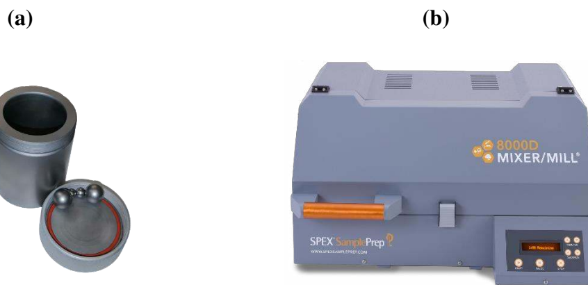
Figure 3.1 (a) Milling vial with stainless steel balls and (b) high energy ball milling device.
