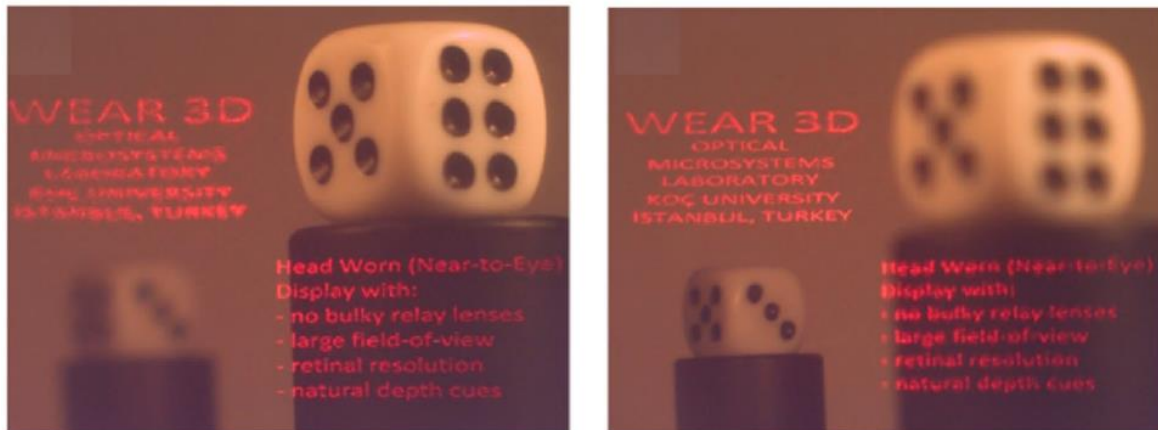
Figure 1.24. Holographic display with 4x4mm eyebox size and 16.7° FOV [68].
