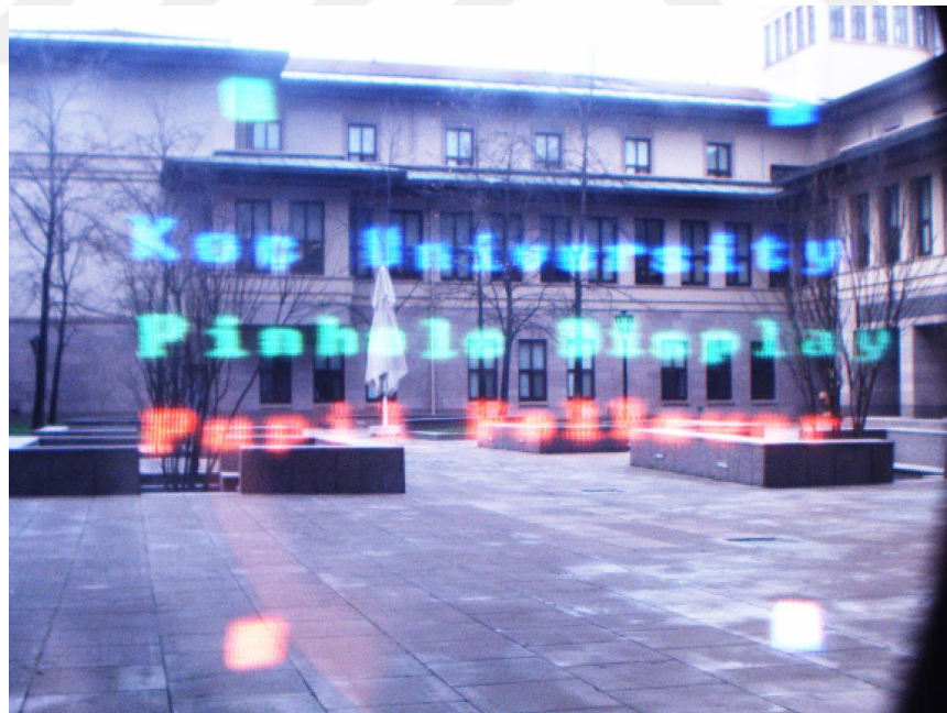
Figure 3.11 Demonstration of the system outdoors. We can show bright images with a single low power LED as all the light is captured by the eye. FOV is roughly circular and 37^\circ .
