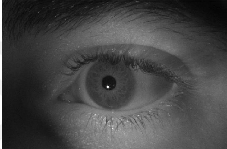
Figure 2.1. The captured image of the eye under IR illumination using a camera with its IR light blocker filter replaced by a visible light blocker.
