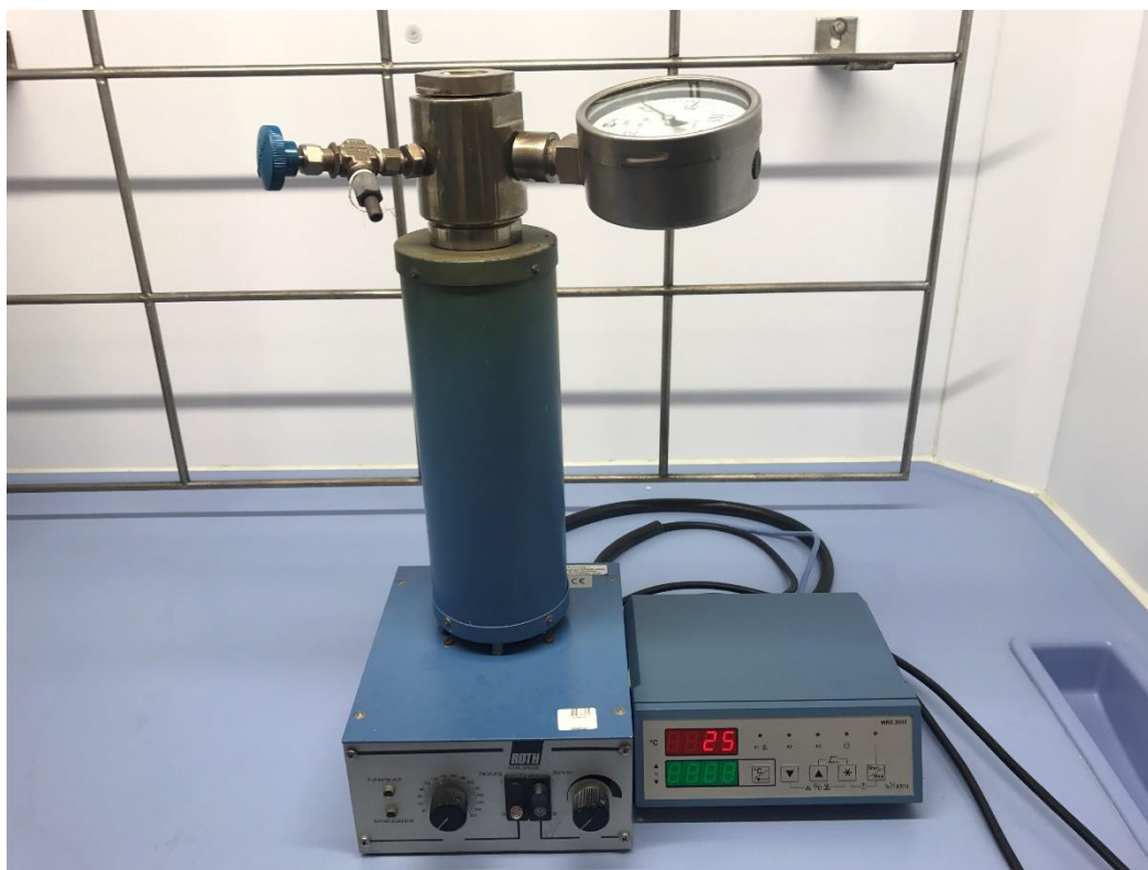
Figure 2.1 Autoclave setup for hydrothermal treatment before modification
