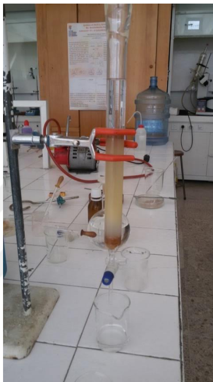
Figure 3.14. Silica gel column chromatographic set-up
