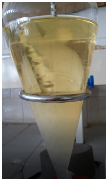
Figure 3.5. Liquid-liquid extractions, separation of ethyl acetate and ethanol
