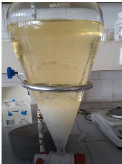
Figure 3.4. Liquid-liquid extractions, separation of chloroform and ethanol
