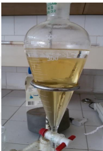
Figure 3.3. Liquid-liquid extractions, separation of petroleum ether and ethanol
