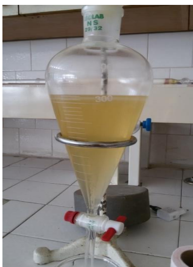
Figure 3.2. Liquid-liquid extractions, separation of hexane and ethanol
