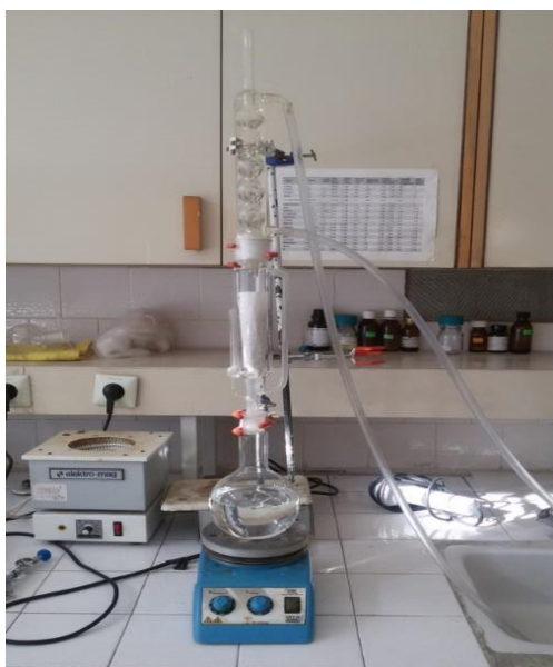
Figure 3.1. Soxhlet extraction setup used for solid-Liquid extraction of amygdalin from powdered bitter almond seed
