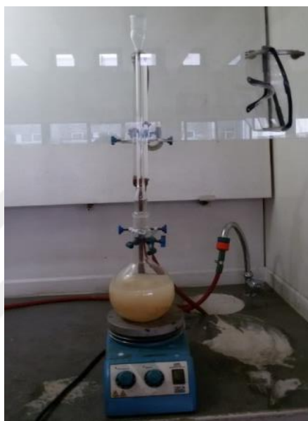
Figure 3.6. Reflux extraction setup used for solid-liquid extraction of amygdalin from powdered bitter almond seed
