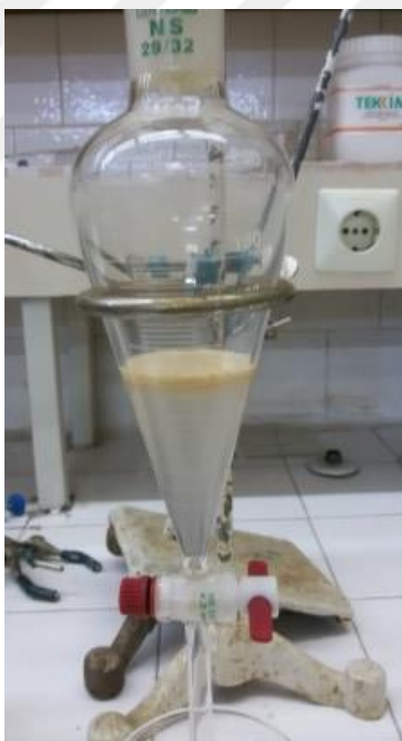
Figure 3.10. Washing precipitate with chloroform
