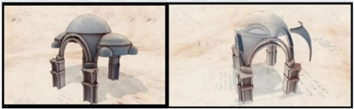
Figure 1.3. The semidomes (on the left) and the pendentives (on the right) [5].
