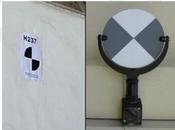
Figure 3.1. The point target (on the left) and the magnetic target (on the right).
