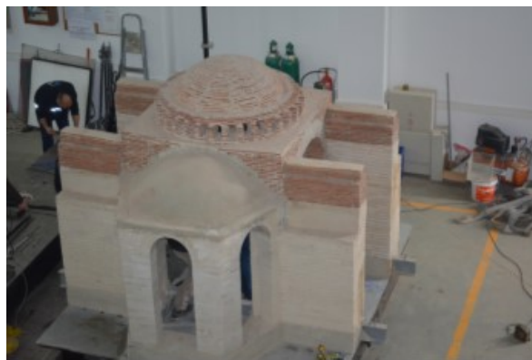
Figure 2.11. Scaled model of Hagia Sophia developed for the shake table test [33].
