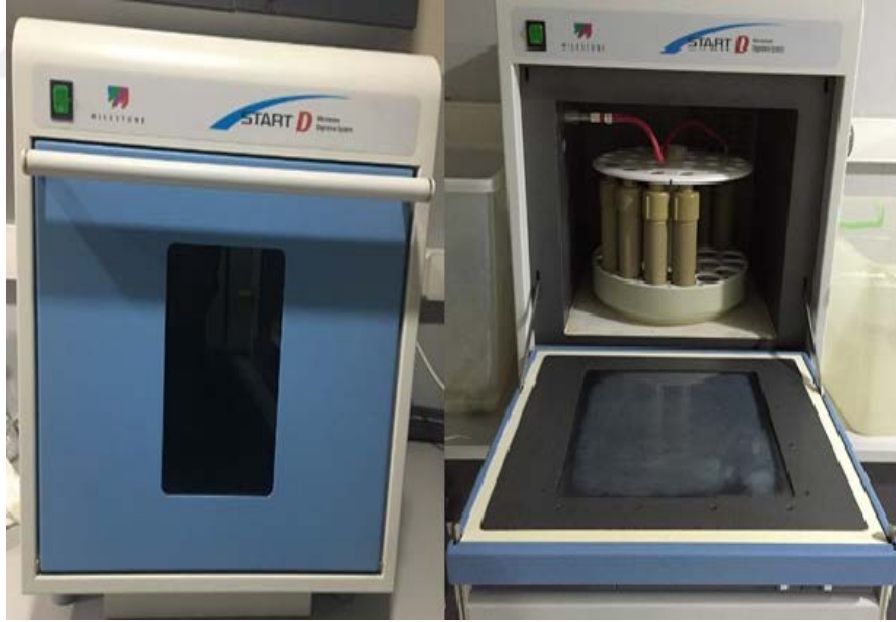
Şekil 3.8: Mikrodalga sistemi (Milestone Start D Microwave Digestion System)
