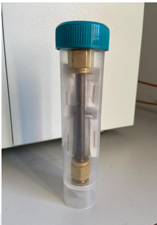
Figure 3.9. Tenax-TA tube and packs of activated carbon and silica gel in falcon tube (photo taken from our laboratory)
