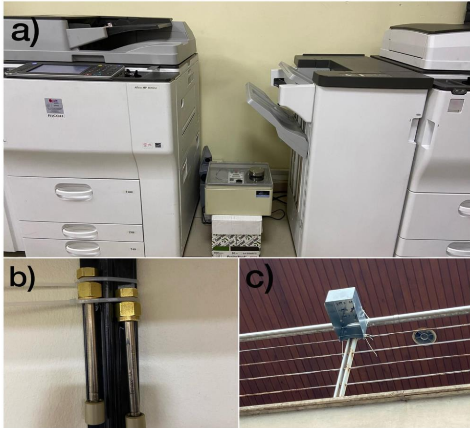
Figure 3.2. a) indoor active sampling, b) indoor passive sampling, and c) outdoor passive sampling in the copy center in the Activity Center of BAIBU
