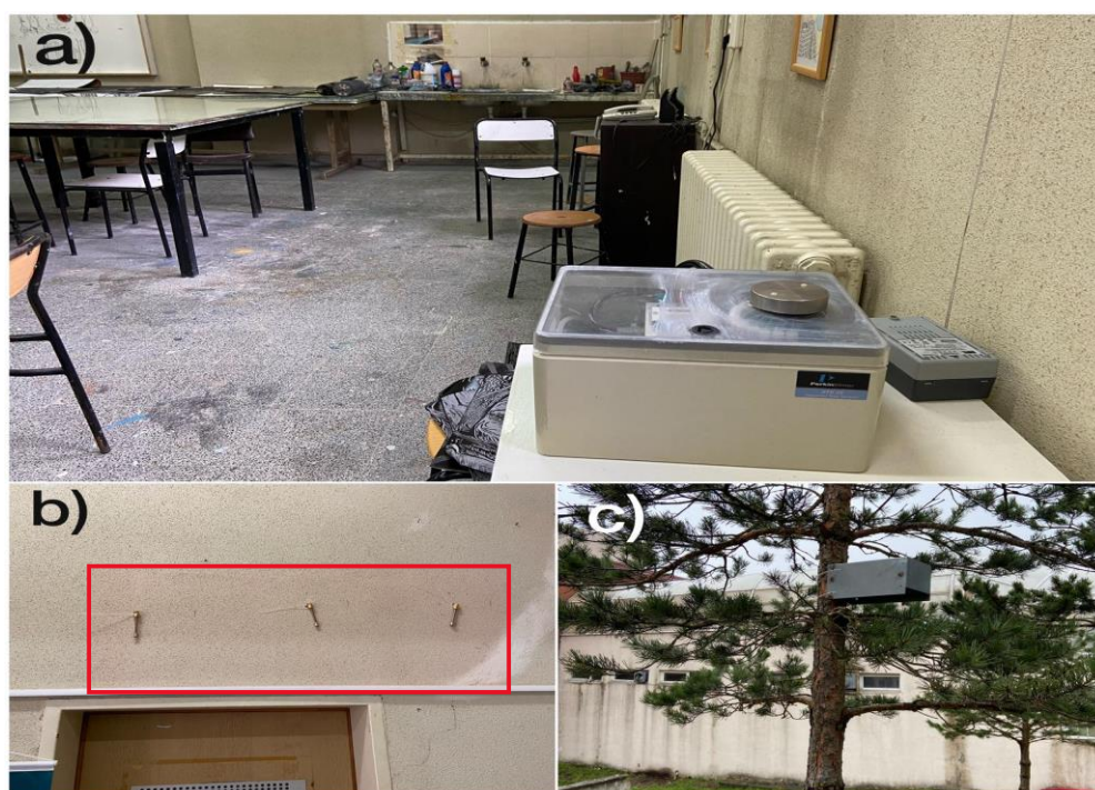
Figure 3.5. a) indoor active sampling, b) indoor passive sampling, and c) outdoor passive sampling in the printmaking class in the BAIBU Faculty of Education
