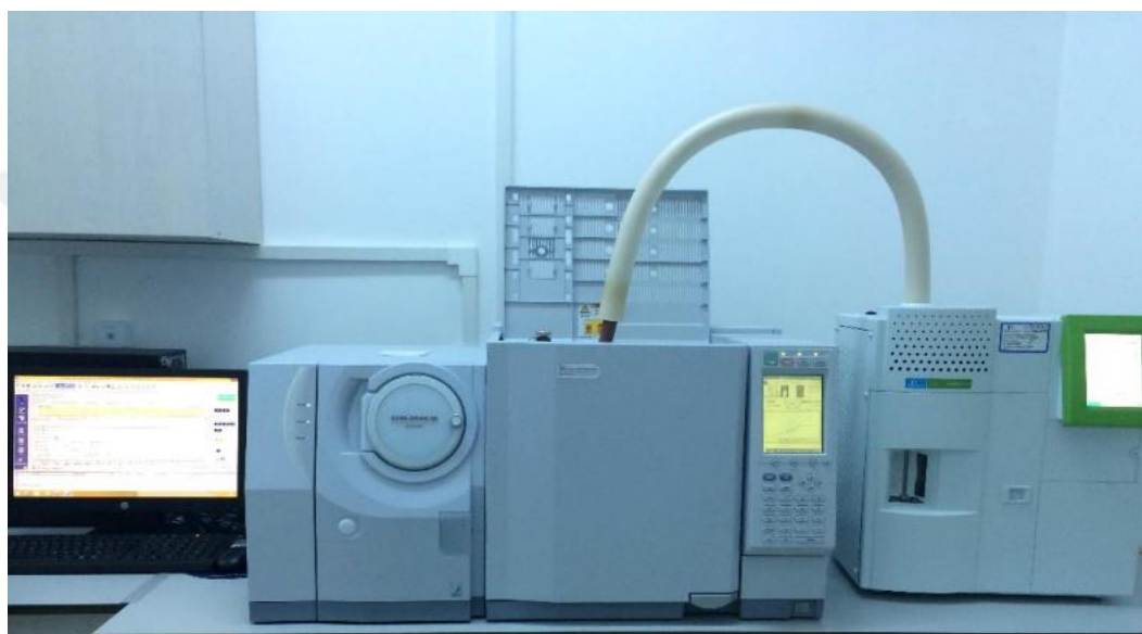
Figure 3.12. The TD-GC-MS system used for VOC analysis (Photo from our laboratory)
