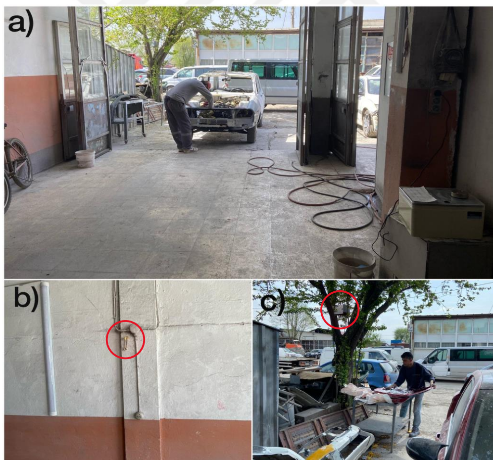
Figure 3.7. a) indoor active sampling, b) indoor passive sampling, and c) outdoor passive sampling in the car painter
