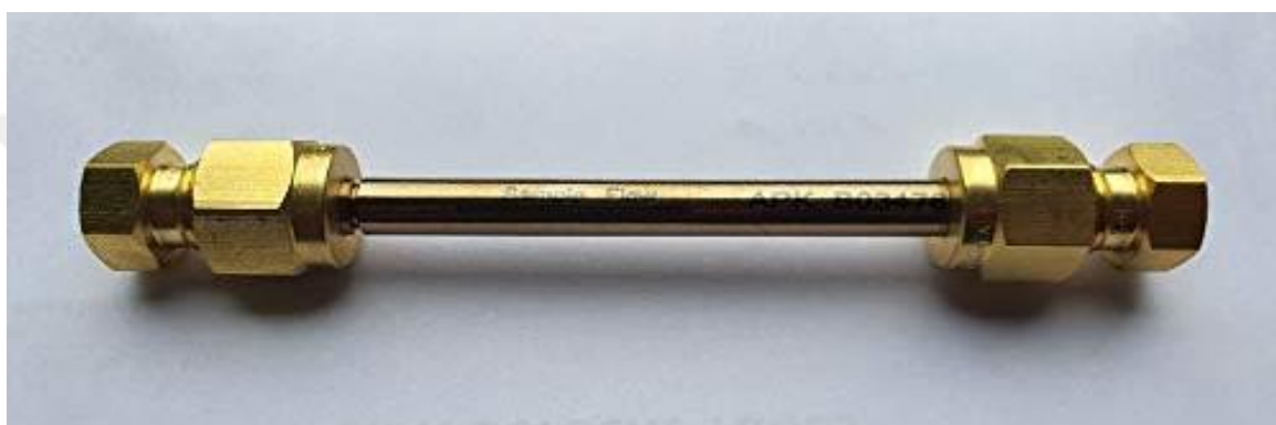
Figure 3.8. Tenax-TA tube used in the active and passive sampling of VOCs (photo taken from our laboratory)
