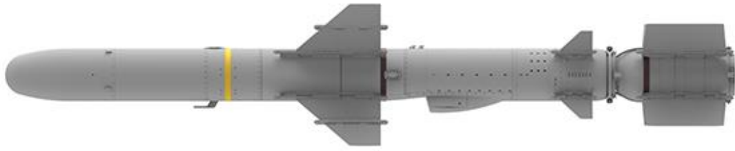
Figure 1.5. Semi-submerged Intake - ATMACA Missile [7]
