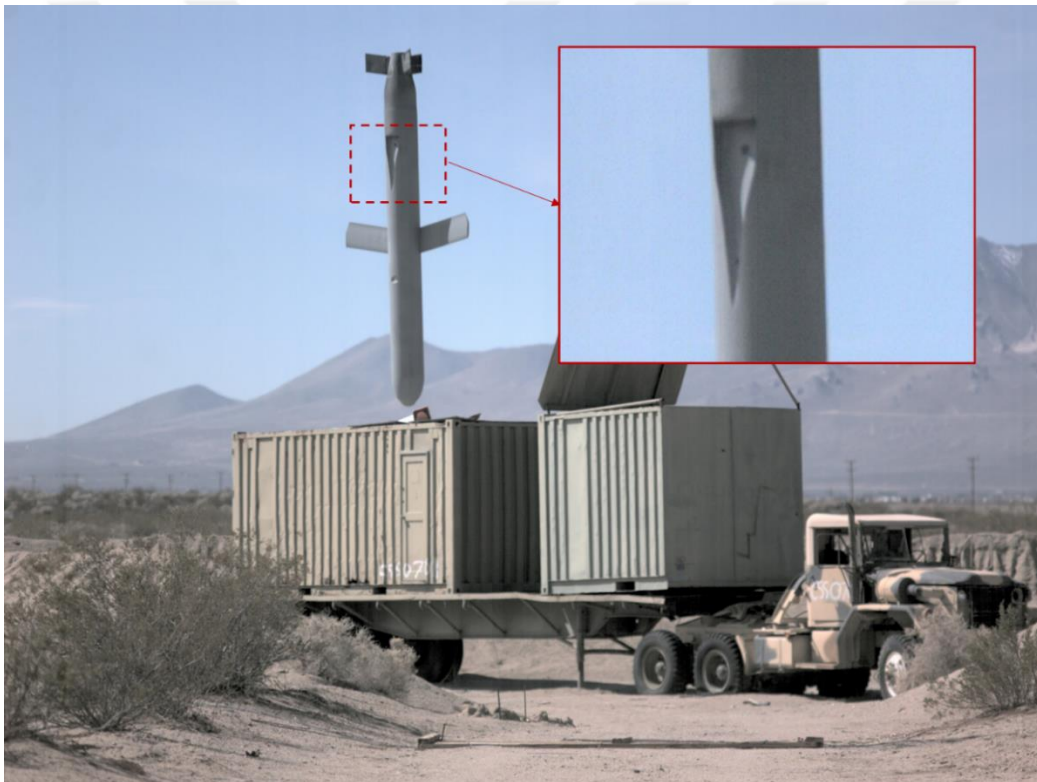
Figure 1.4. Submerged Intake - Tomahawk Missile [6]
