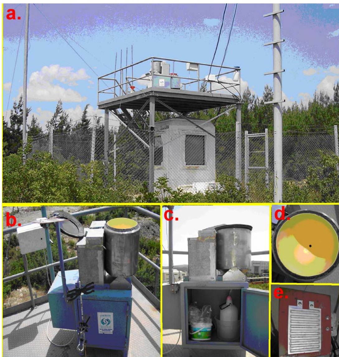
Figure 3.1 (a) General view of Tinaztepe sampling platform, (b) and (c) general perspectives of automated sampler, (d) plastic collection funnel of sampler, (e) rain sensor of sampler.
