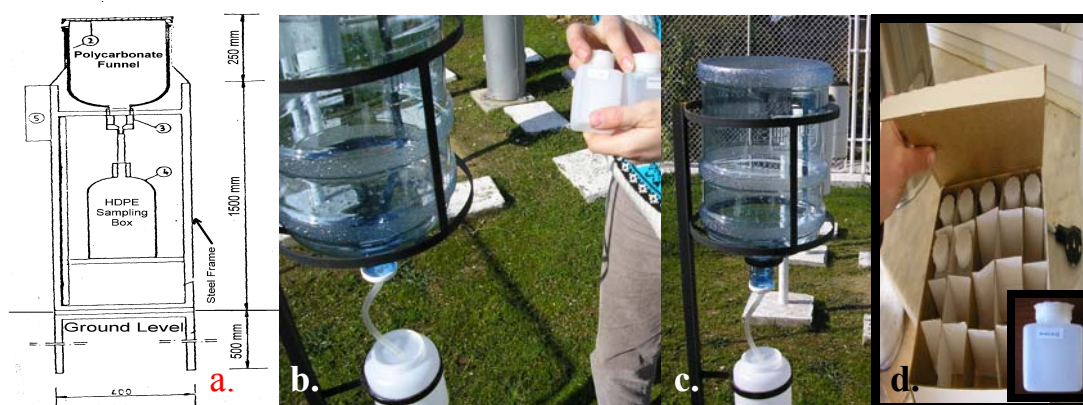
Figure 3.2 (a) Schematic view of manual sampling equipments, (b) and (c) general views of manual sampling equipments located in meteorological observation parks, (d) storing of sampling bottles.
