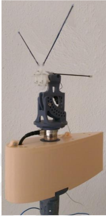
Figure 3.12: Flapping wing mechanism without the wing skin
