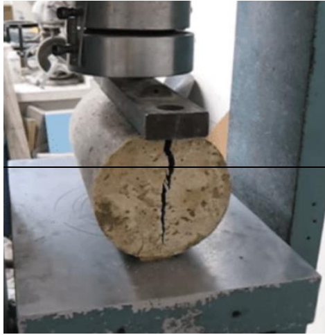
Figure 7. Split Tensile Test (Gundaraniya, 2022)
