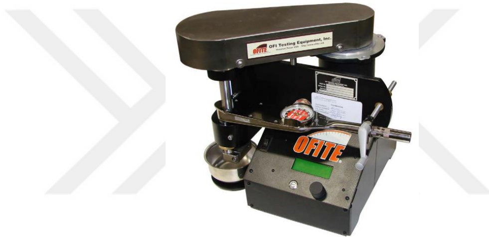
Figure C-1. Lubricity Tester (OFITE Instruments, 2015)
