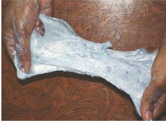
Figure 2.7. Stiff Rubbery Gel After Complete Gelation (Suyan et al, 2007)
