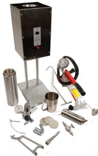
Figure B-1. Permeability Plugging Apparatus (FANN Instruments, 2016)
