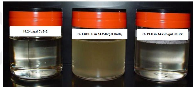
Figure 2.2. Lubricants shown in 14.2-lb/gal after 3 hr at 215°F. Lube C has been used for many years in reservoir drilling fluids. Typical concentration for PLC is 0.6 vol % (Foxenberg et al, 2008)
