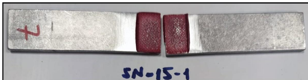
Figure 5.11: The real image of interface of the 15mm overlap Single Lap Joint specimen which were ruptured after 3 shots in the experiment.
