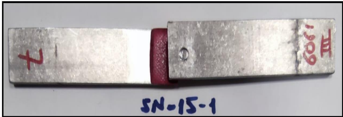
Figure 5.12: The real image of front side of the 15mm overlap Single Lap Joint specimen which were ruptured after 3 shots in the experiment.
