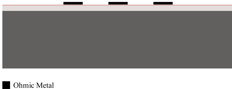
Figure 2.3: The cross-section of the structure after the alloyed ohmic contact process.
