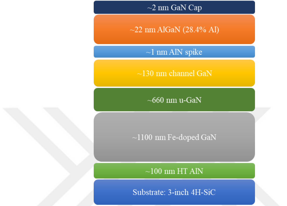
Figure 2.1: Epitaxial structure showing the layers grown by MOCVD.
