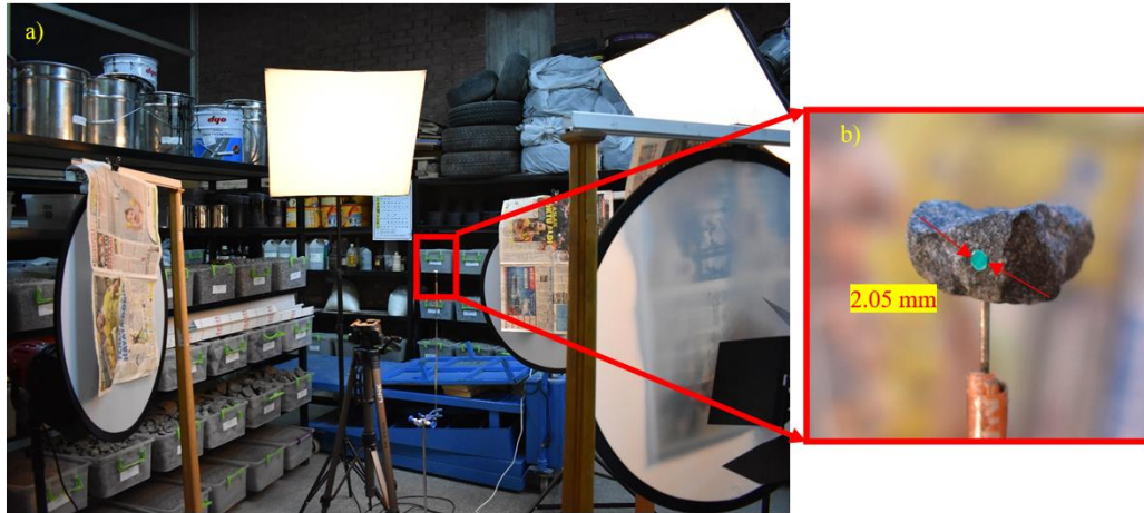
Figure 16 3D photogrammetry setup a) setup b) aggregate
