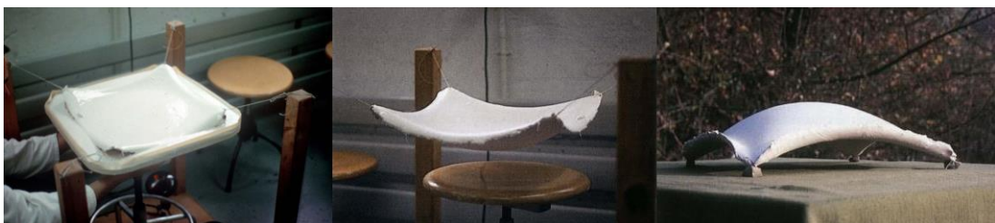
Figure 4.5 Stage 1: Dipping the cloth into a hardening substance. Stage 2: Hanging the model Stage 3: Inverting the hardened model (John Chilton 2000)
