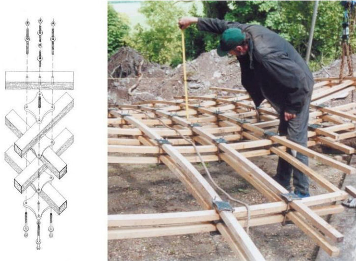
Figure 4.53 Gridshell Detail (Buro Happold/ Adam Wilson)
