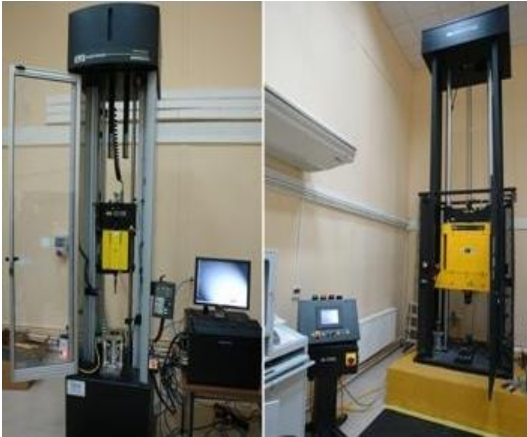
Figure 2.6 : INSTRON 8150 Drop Test Machine [18].
