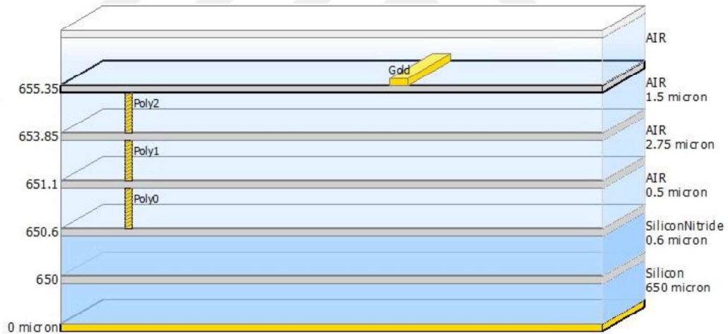
Figure 3.7. Constructed stack in ADS
