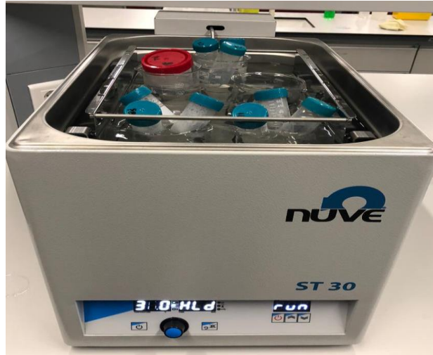
Figure 3.6. Shaking water bath with nanocomposite formulations
