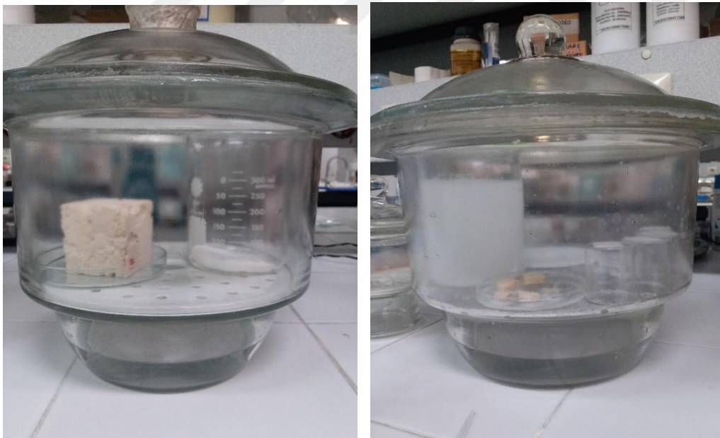
Figure 20. Representation of carbonation process of dolomite samples in desiccator with high RH and high \text{CO}_2 partial pressure.
