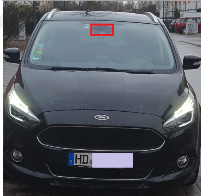
Figure 3.1. Front camera installed on a car
