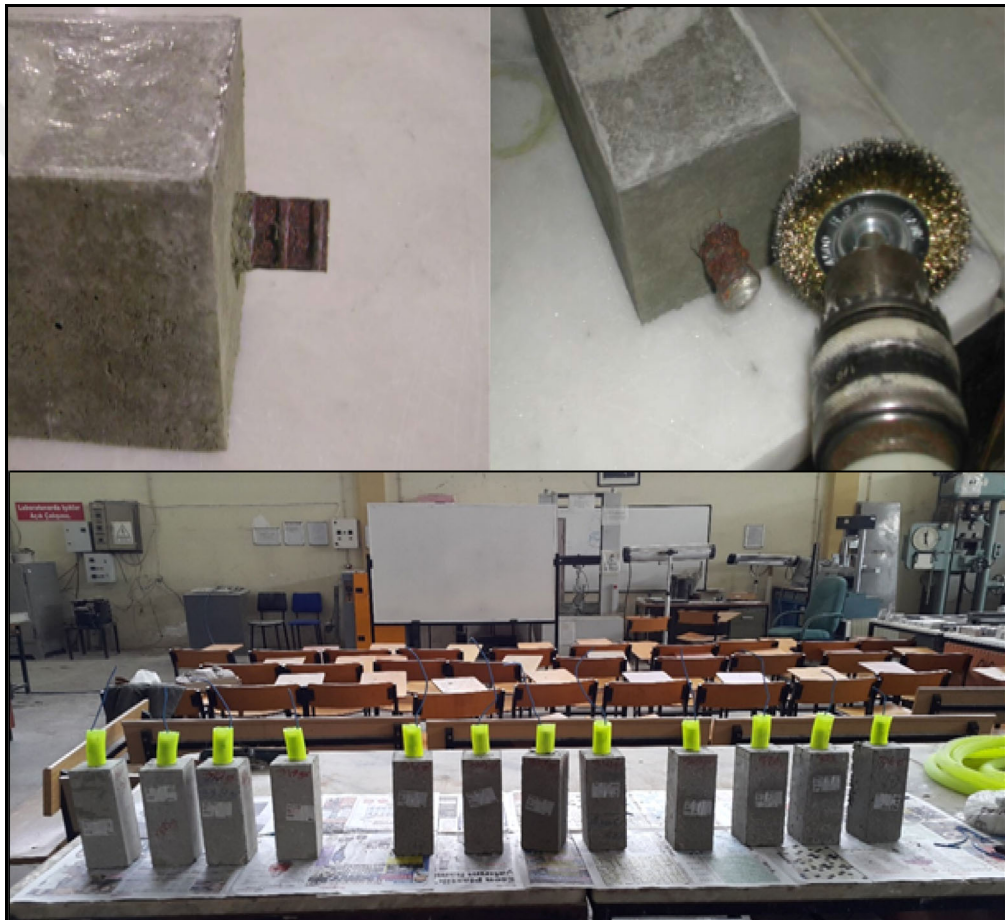
Figure 3.6 Rust cleaning before preparing samples (Personal archive, 2016)
