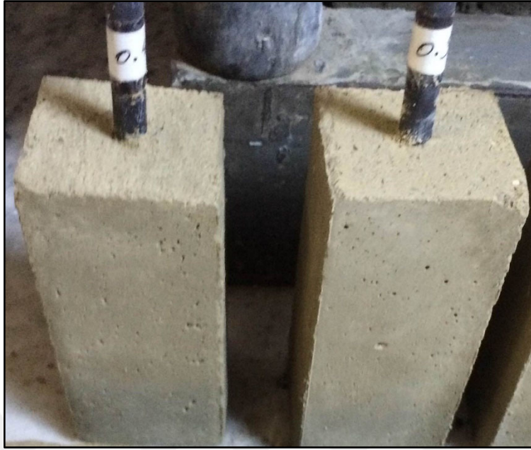
Figure 3.10 Reinforced concrete specimens (Personal archive, 2016)
