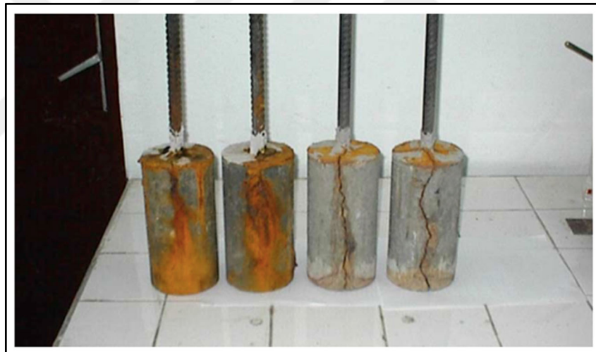
Figure 2.11 Specimens after corrosion test (Guneyisi, et al., 2009)
