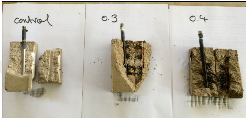
Figure 4.12 Steel reinforcement after electrochemical tests (Personal archive, 2016)
