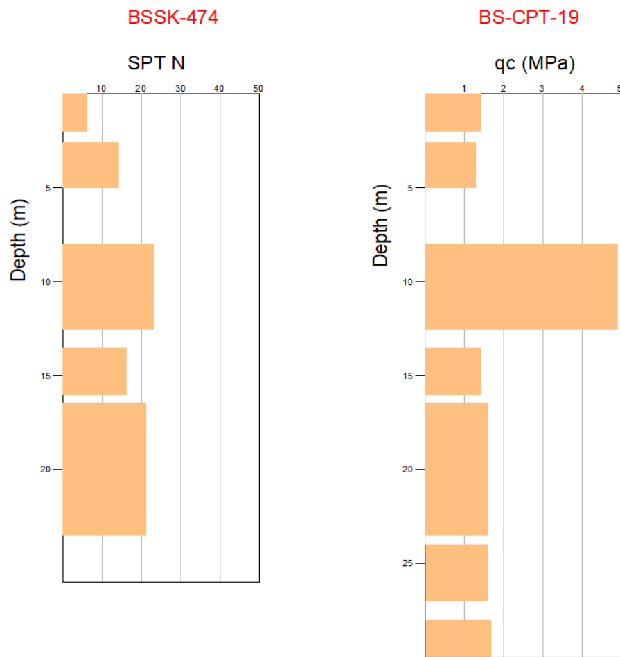
Figure 3.68. SPT N vs. Depth (m) and q_c (MPa) vs. Depth (m) graphs for clay layers
