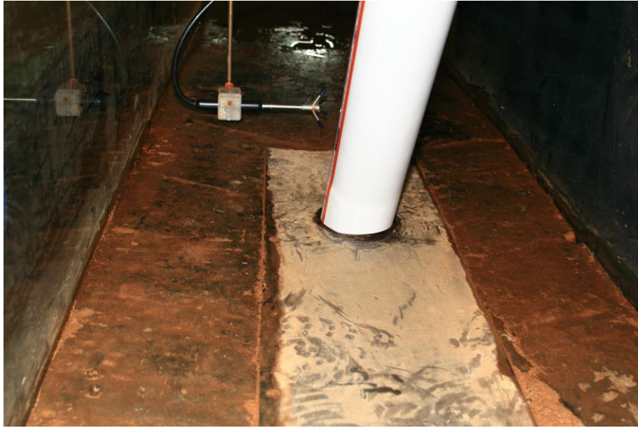
Figure 3.3 : Mounted obstacle pier and ADV probe.
