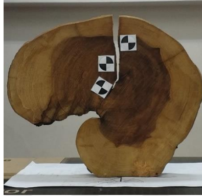
Figure 5.12. Wooden Specimen Used in Case Study-2
