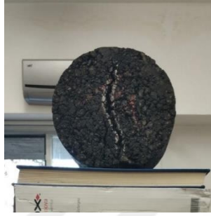
Figure 4.1. Cracked Asphalt Specimen
