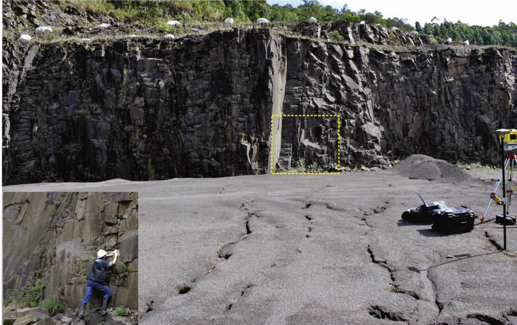
Figure 1.2. TLS data acquisition of a basalt quarry, Gomes et al. (2016).
