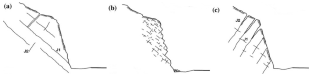
Figure 1.1. Effects of discontinuity orientation on slope stability. (a) Persistent J1 discontinuities dipping out of face forms potentially unstable sliding blocks, (b) closely spaced, low persistence discontinuities cause ravelling of small blocks, (c) persistent J2 discontinuities dipping into face form potential toppling slabs, Wyllie and Mah (2004).
