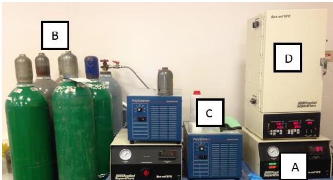
Figure 16. Supercritical Drying Unit from Applied Separations™
