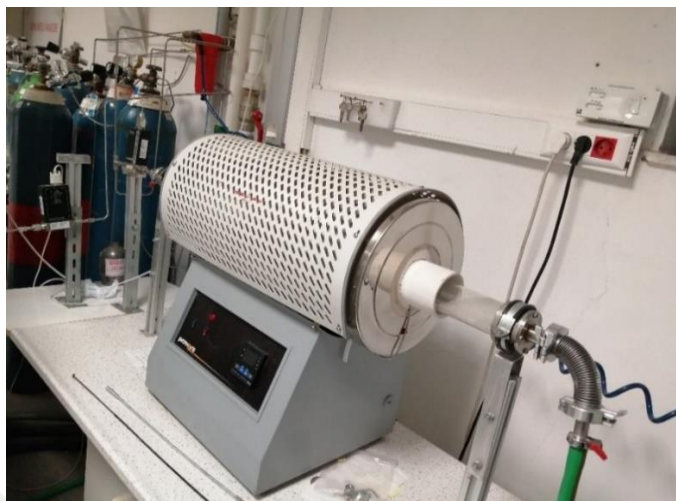
Figure 13. Tube furnace used in the pretreatment protocols.
