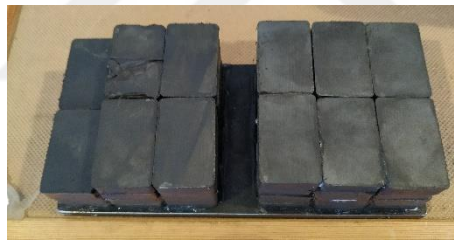
Figure 5.2 The test magnetic circuit with broken magnet (Personal archive, 2019)
