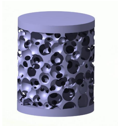
Figure 13: Final cellular structure with 0.2 relative density block after extraction
