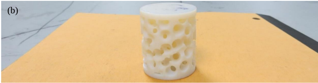
Figure 37: Stress-strain curve (a) and the AM manufactured cellular structure (b) for \rho = 0.35
