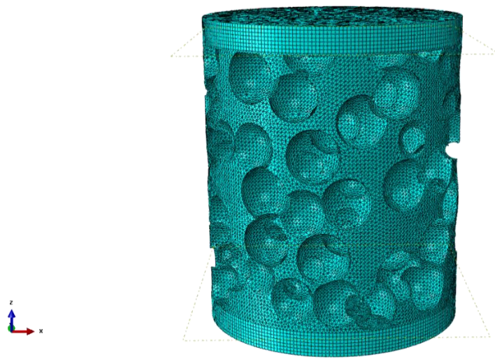
Figure 14: Cellular structure with 0.4 relative density block meshing
