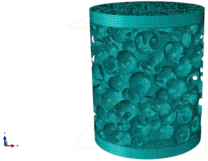
Figure 18: Cellular structure with 0.2 relative density block meshing
