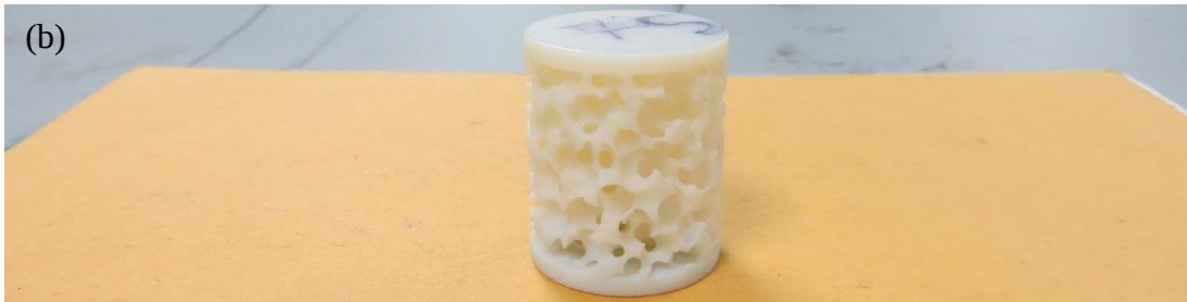
Figure 39: Stress-strain curve (a) and the AM manufactured cellular structure (b) for \rho = 0.25
