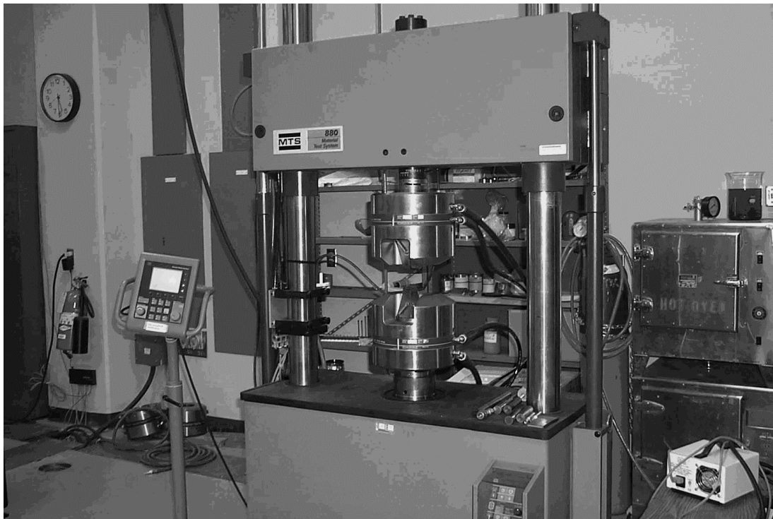
Figure 35: MTS 880 system for compression test.
