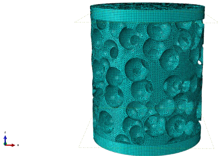
Figure 15: Cellular structure with 0.35 relative density block meshing
