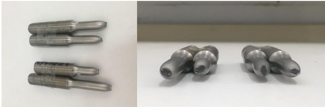
Figure 5.7. Broken tensile test specimens prepared from base metal region of X70 steel
