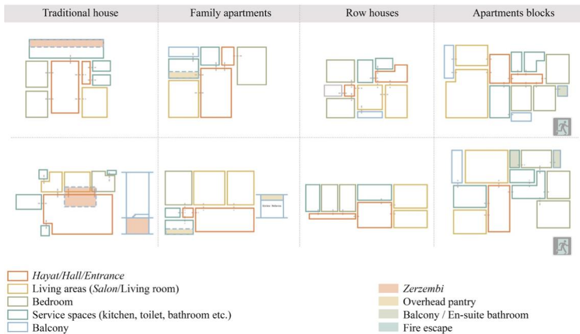
Figure 5.12 The re-signification of zerzembi (storage space)
