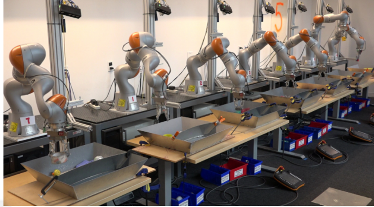
Figure 3.6: Large-scale robotic grasping data collection. [Kalashnikov et al., 2018] describes how a dataset of over 500,000 grasp trials collected from multiple robots was used to train a vision-based grasping policy, comparing fully offline training and online fine-tuning.
