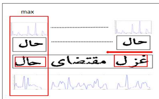
Figure 2.10: A query word is searched in a candidate line by a sliding window approach and at each iteration, matching score is calculated for query word and the generated source pseudo-word.
