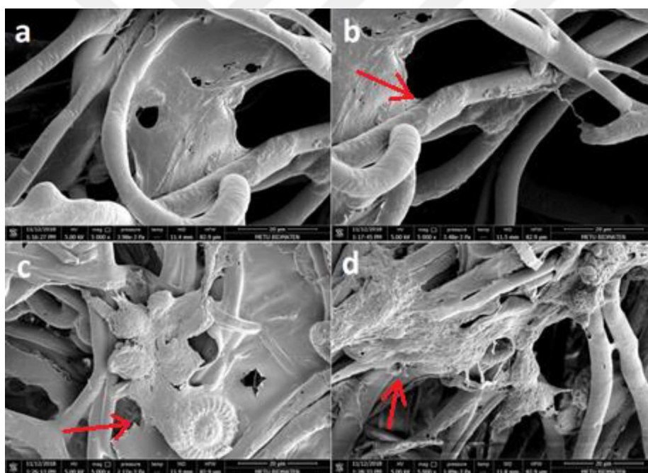
Figure 3.33. SEM images of Saos-2 cells proliferating for 7 days on B-PHBV/PCL (a and b) and B-PHBV/PCL/CA:PUL/DS (c and d) scaffold groups. (Arrows: Cells on fibers). The scale bars on the images show 20 \mu\text{m} length.
