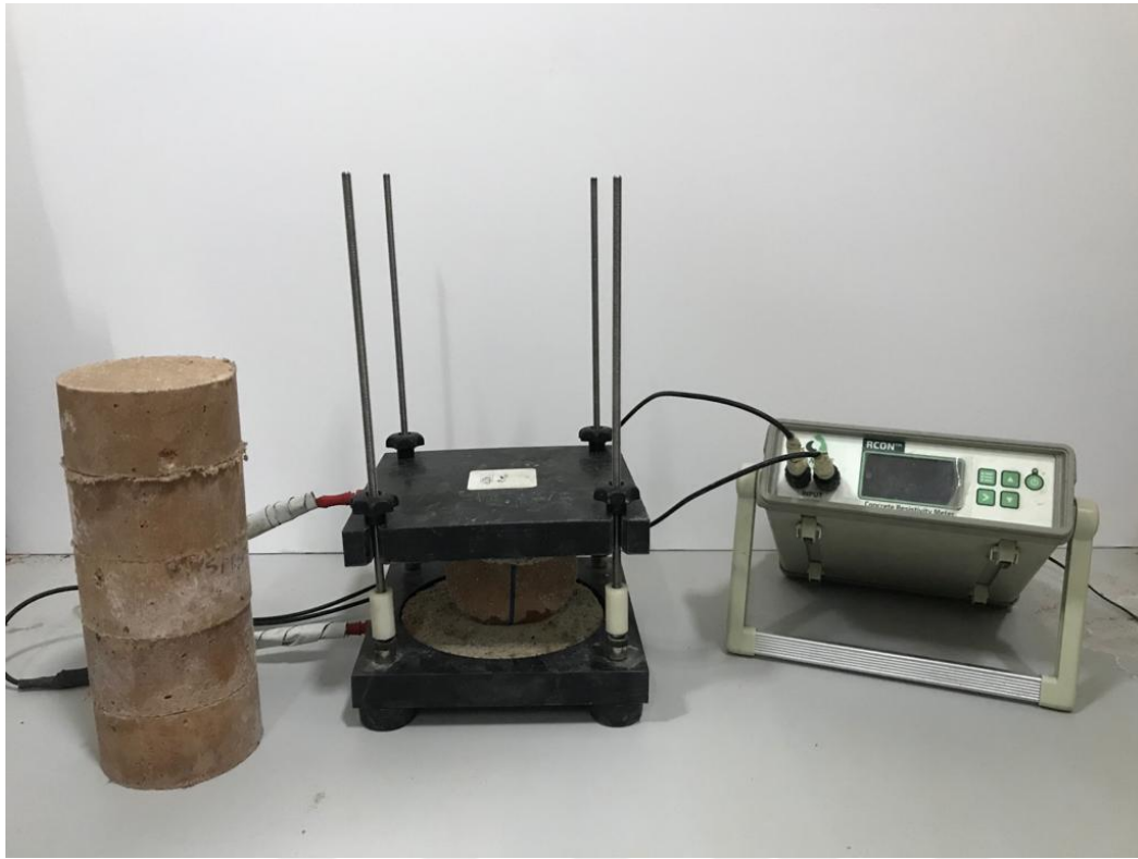
Figure 3.12. Electrical impedance testing device
