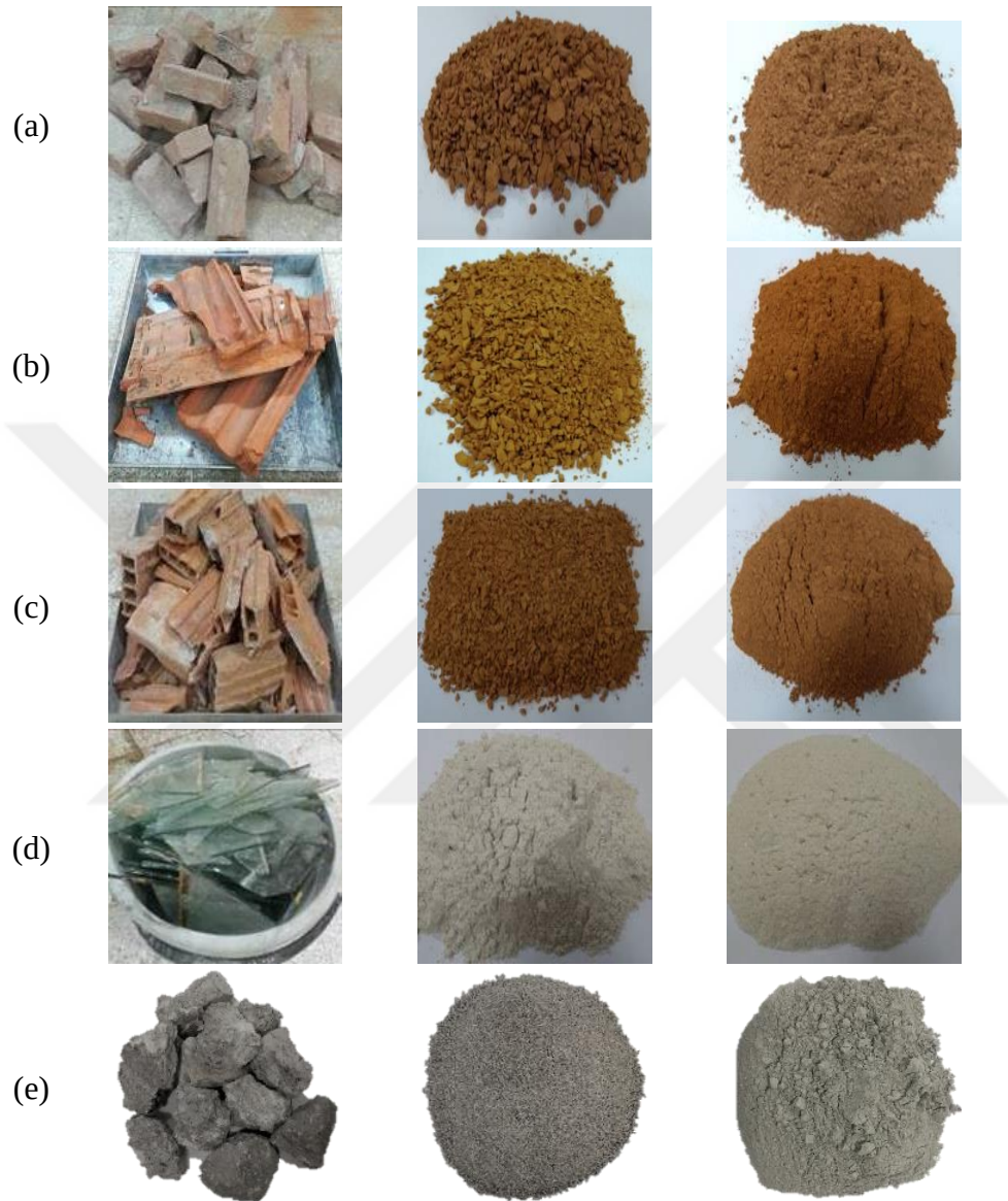
Figure 3.1. CDW-based materials in bulk, crushed and ground form red clay brick (a), roof tile (b), hollow brick (c), glass waste (d), concrete waste (e)
