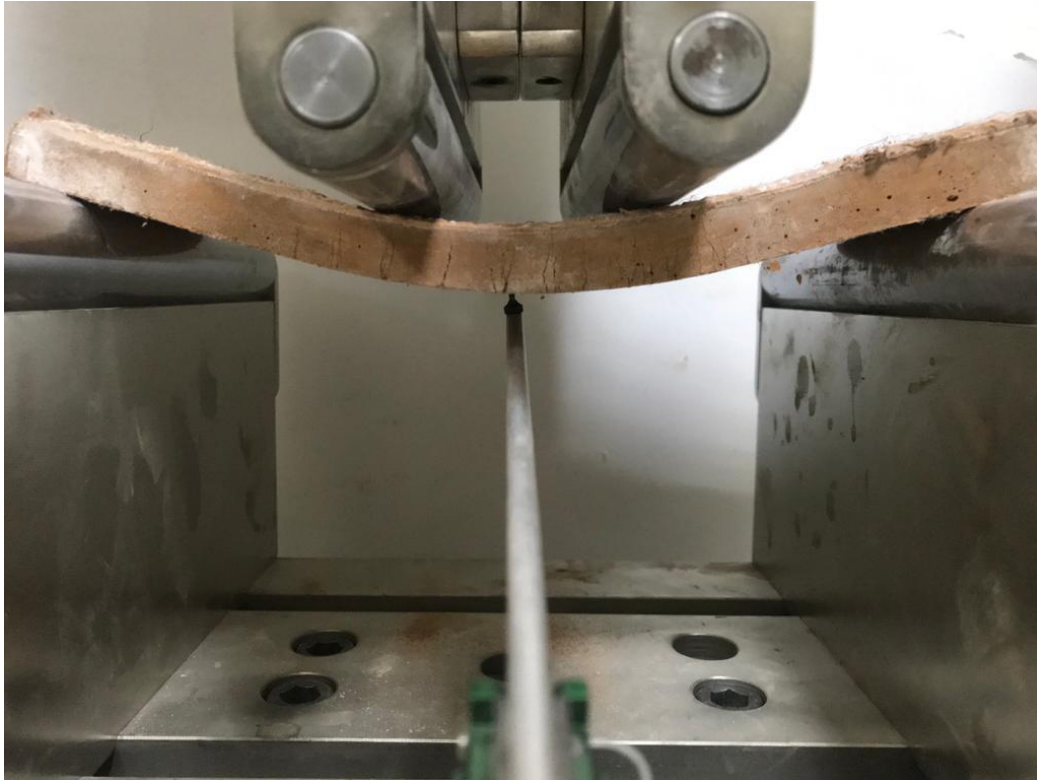
Figure 3.14. Midpoint displacement recording with deflectometer
