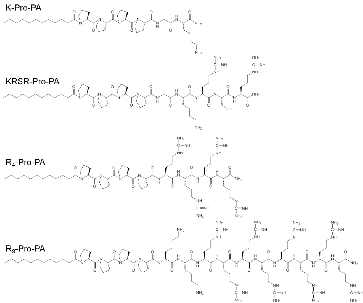
Figure 4.1. Chemical structures of PAs that are used in this study: C 12 -P 4 GK (K-Pro-PA), C 12 -P 4 GKRSR (KR SR-Pro-PA), C 12 -P 4 R 4 (R 4 -Pro-PA) and C 12 -P 4 K 2 R 8 (R 8 -Pro-PA).
