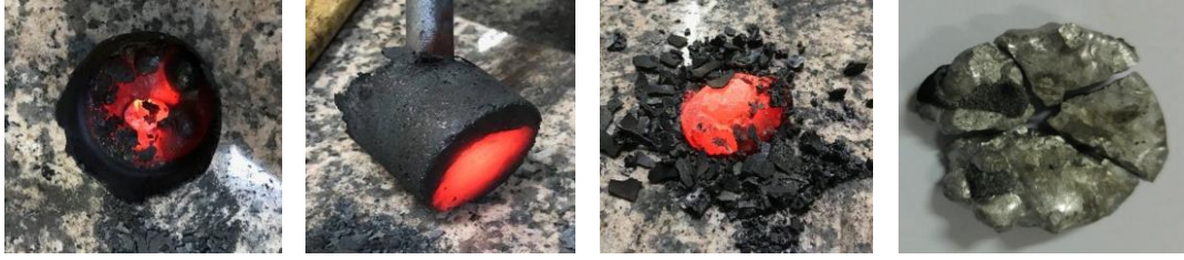
Figure 5.2 The images of obtained product as a result of SHS experiments
