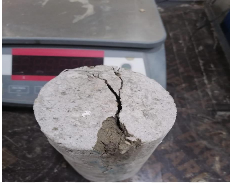
Figure 3.12: Splitting Test Result.
