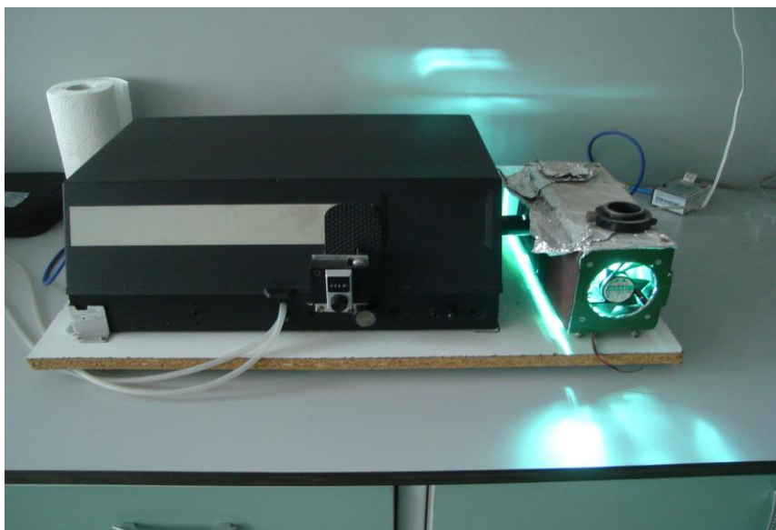
Figure 5.1: A handmade UV-absorbance spectrometer.
