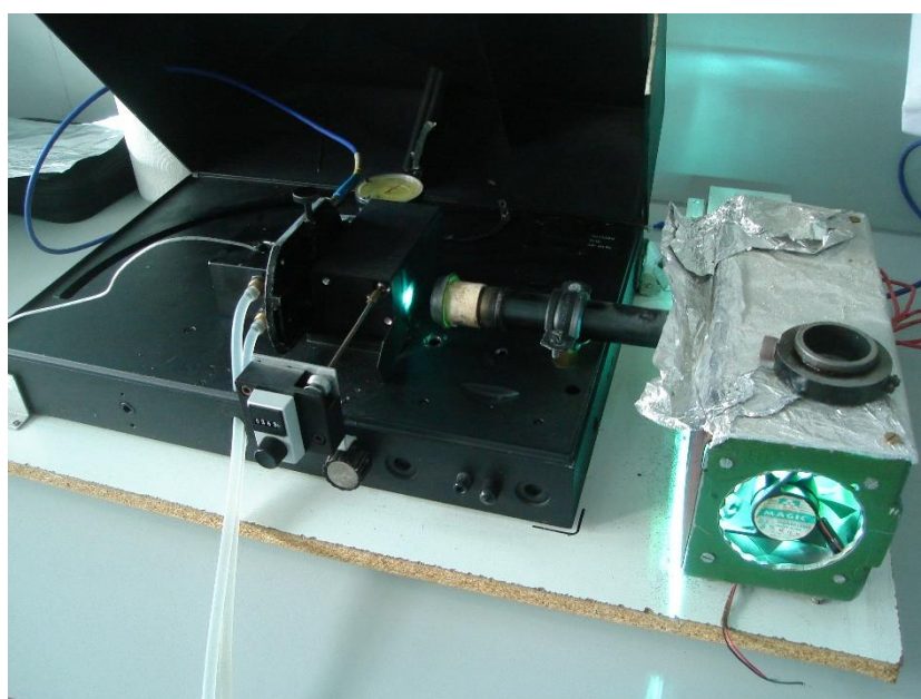
Figure 5.2: The open-view of the UV-absorbance spectrometer.
