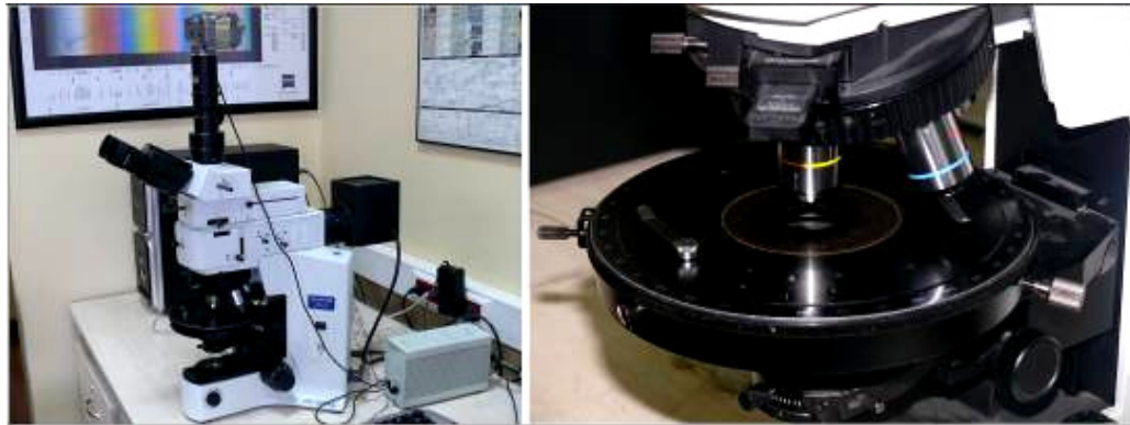
Figure 2.5 Olympus BX41 binocular polarizing microscope with a high intensity 6V, 30W halogen light source combined with U-CPA and U-OPA optical systems, used in this investigation.
