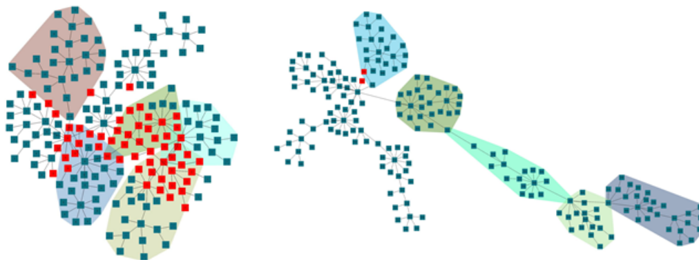
Figure 4.7: A real life graph of 242 nodes, based on gondola gene data laid out with CoSE (left) and Cluster Layout (right) [19]
