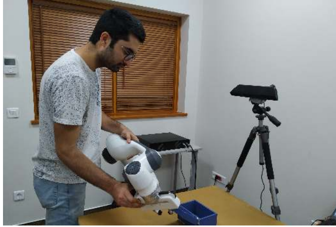
Figure 3.3: User kinesthetically teaches close the box skill to Franka Emika Panda arm. Microsoft Kinect V1 records Point Cloud data of the object of interest.
