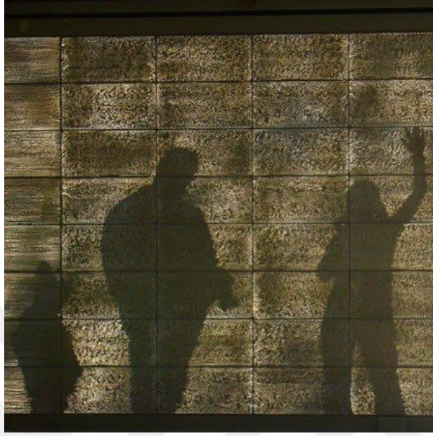
Şekil 4.18. LitraCon (light transparent concrete), Aron Losonczı, 2002 (URL-20)
